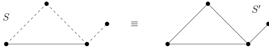
Figure 3.2: Signed graph S is switching equivalent to an all-positive signed graph S'
